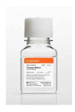
Corning Transport Medium is an isotonic solution at neutral pH containing protective proteins, an antibiotic to prevent microbial growth, and an anti-mycotic to prevent contamination by yeast
